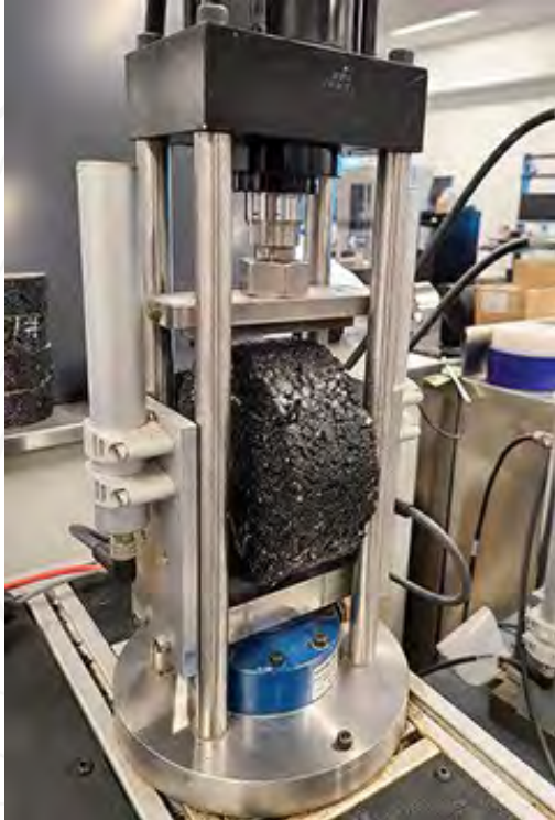
The mixtures placed in the field projects are tested via the ideal cracking test in the CIR Asphalt Innovation Laboratory.
